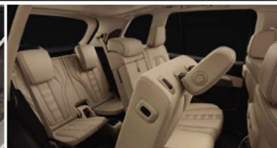
3 rd row seats with 2 nd row of seats incl. comfort entry and infinitely variable electric seat backrest tilt adjustment and fore-and aft adjustment incl. Comfort cushions.
